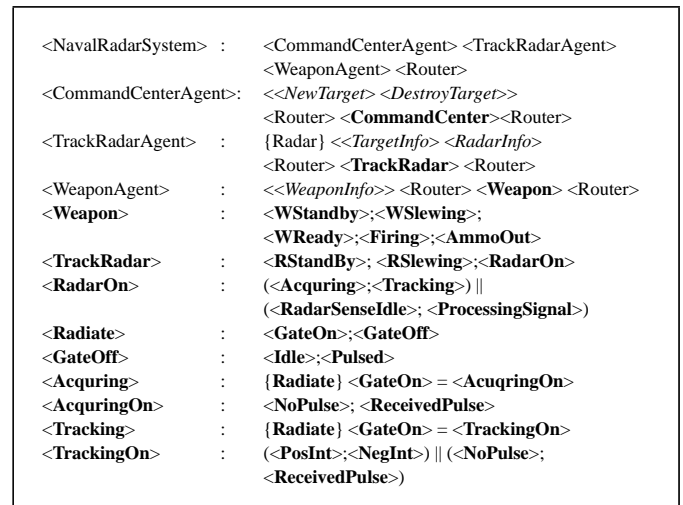
Figure 4. High-level System Specification
